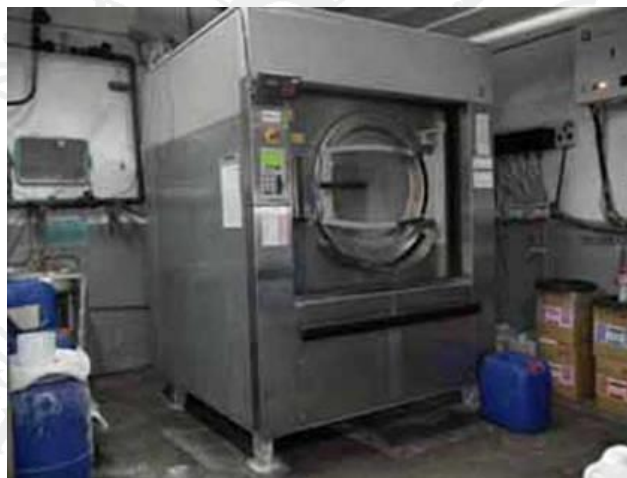
Figure 2.10 Large washing machine using ozone system for water- and chemical – saving washing
